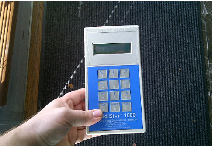
FieldStar 1000 Gaussmeter used during EMF/EMC Study
