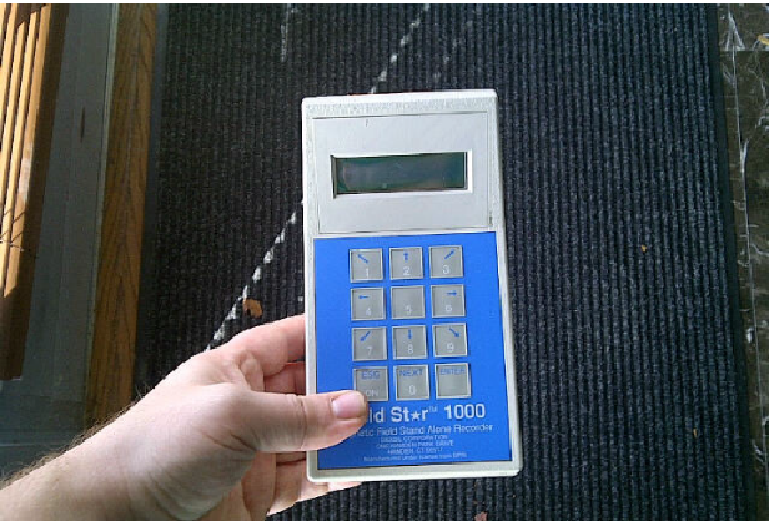
FieldStar 1000 Gaussmeter used during EMF/EMC Study
