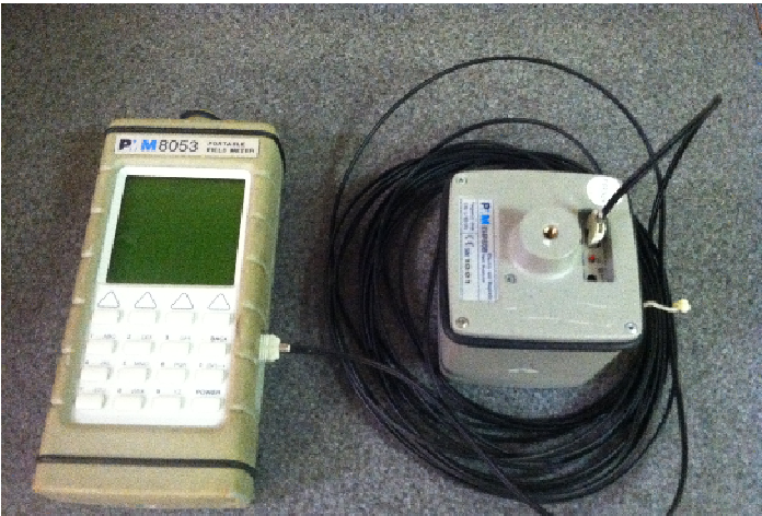
PMM 8053 3-Axis field meter used to take electric field readings
